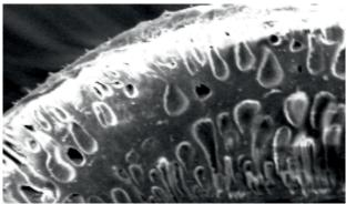
SEM micrographs of hollow fibers showing double active layer
