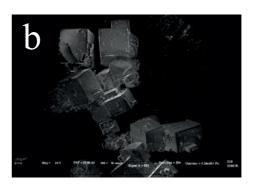
(a) Optical microscopic image of NaCl cubes and (b) corresponding SEM image showing agglomerated nearly perfect NaCl cubes
