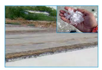
Left: Demonstration of low sodium salt technology to M/s. HUL at Tuticorin, Tamil Nadu Right: Carnallite getting crystallized in the solar pans
