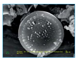
Mesoporous carbon-celite 545 template image showing the formation of mesoporous carbon inside the celite 545 template
