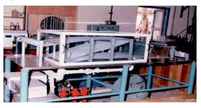
Casting machine for making heterogeneous membranes
