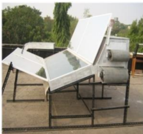
Indirect natural convection solar dryer (left) and reduction of moisture with time (right)
