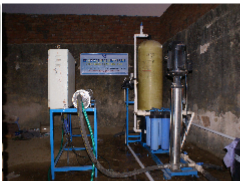
Inauguration (extreme left) of 2500 LPH plant was setup in partnership with DST and Rajasthan State Science and Technology, September, 2010, Theekariakalan village, Nagaur-Dist., Rajasthan. Feed :10,000 ppm; Product water :300 ppm (Left) and Siripuram village, Nalgonda district, AP (August 2009) 4000 LPH plant set up with DST and AP State Council support for removal of brackishness and fluoride (Right)
