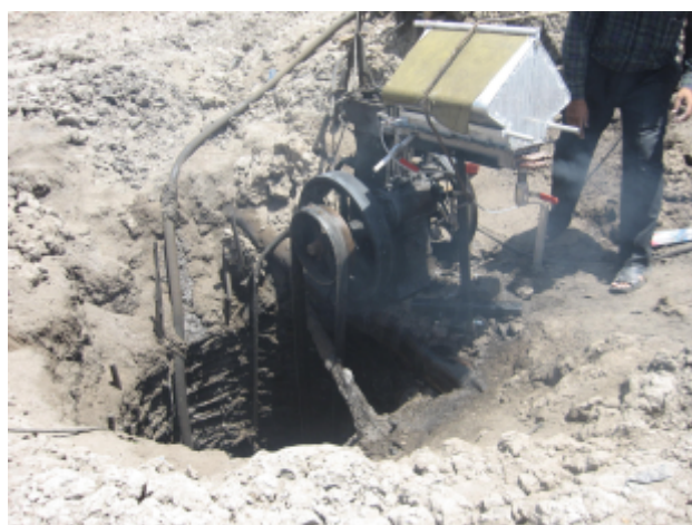
A unit to produce drinking water by desalination of sub-soil brine utilizing waste heat from diesel engine
