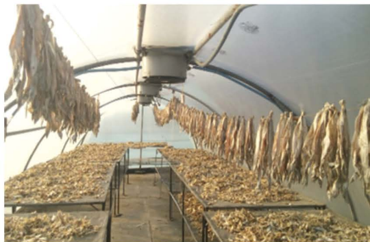
Fig. : Fish being dried inside the constructed solar thermal dryer at Sagar island
