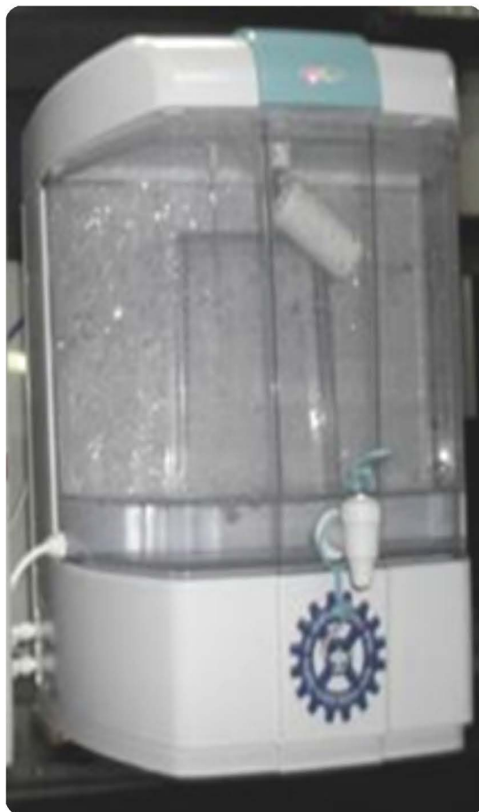
Figs. : Hybrid ED-RO unit for water desalination/purification
