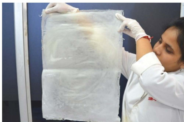
Fig. : Indigenously developed 2-Acrylamido-2-methyl-1-propanesulfonic acid grafted PVDF-co-HFP (SCP-13) based cation-exchange membrane
