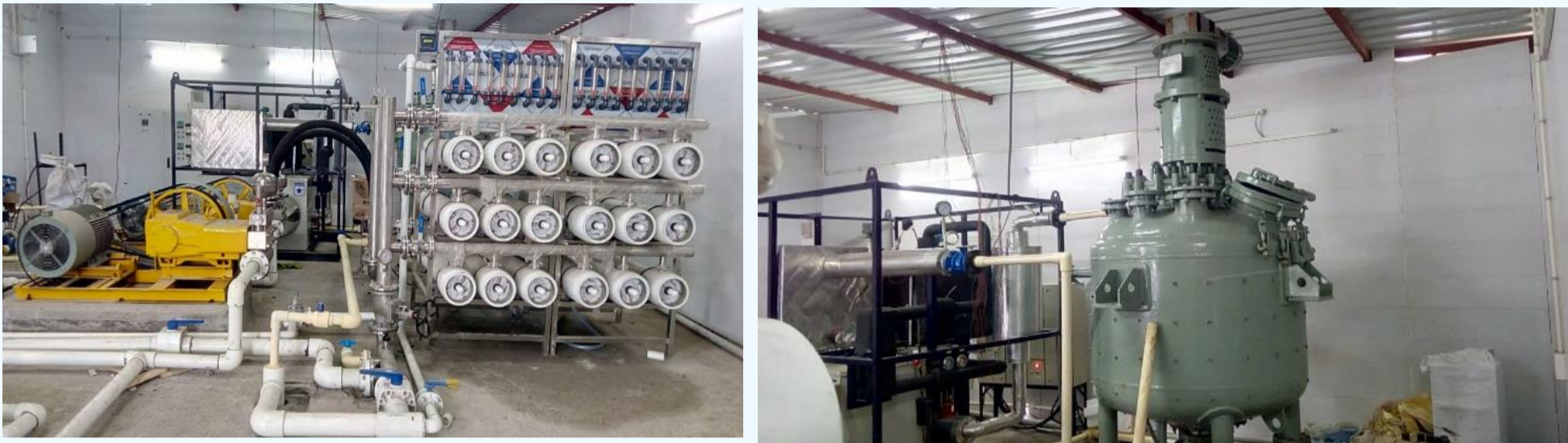
Pilot plant facility established for end-of-life Reverse Osmosis membrane rejuvenation Funding support: Department of Science and Technology India
